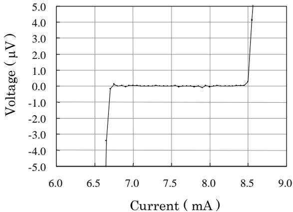
Fig. 1. A current step for an 8-bit DAC at 12.0 K.
